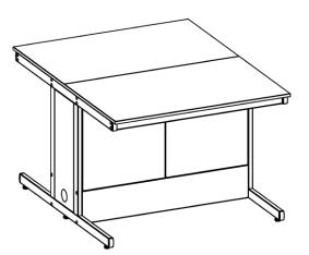
All island tables have special plugs, located in the section supports (both right and left), designed to supply the necessary services.
