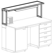
All racks in the Inova series are equipped with fluorescent lights with screens. Power is supplied from a terminal box, which is part of the table elements.
