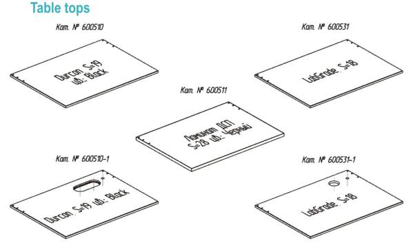
Table tops made of laminated chipboard have durable plastic edge of 2mm thick.
