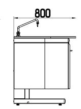
The service compartment takes the entire volume under the washer, thereby providing excellent access to services. Storage compartments are located on the right and left of the door, in aprons.
