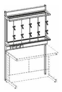
Titration rack complete with a side table is designed to perform various analyses by direct or back titration.
