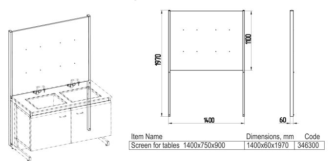
The screen consists of two vertical supports and the box with stiffeners. The box comprises 8 holes with plugs for mounting the wall dryers. "METALLDESIGN" factory produces screens for side tables of 750mmheight as well.
