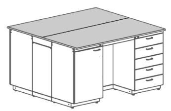
Table tops of island tables are joined together out of two side table tops. Table tops can be combined at will, but be careful: when joining LabGrade and Durcon table tops with laminate ones, the ledge of 10mm thick between different table tops unavoidable.
