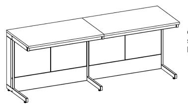
All side and island tables are equipped with height adjustable supports, allowing to set sheerly horizontal working surface.
