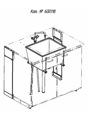
Components of tables with sinks, in addition to screens, fasteners and ties include drain sinks with sanitary equipment and mixer taps with flexible connections.
