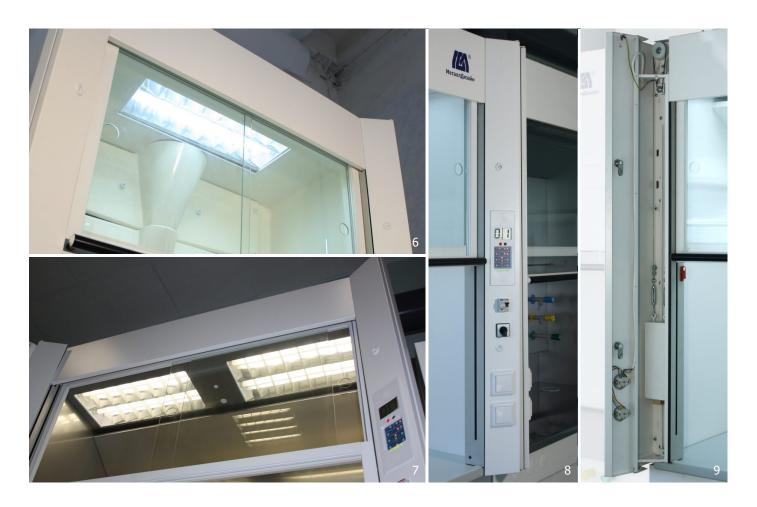
to provide a uniform motion of the sliding screen. The weight is located in the left column of the portal (Pic. 9). All parts (weight, cable in polyethylene housing, rollers) are accessible for maintenance and repair directly from the front side of the hood. It is particularly important if the hood is located in a corner of the room or situated in a single row with other exhaust hoods.
